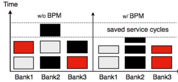
Figure 3. The comparison between interleaved address mapping and BPM. Different colors represent requests from different threads.
