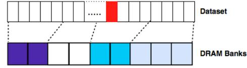
Figure 13. Thread level coloring. The above array is mapped to different bank colors. The colored rectangle in dataset represents shared data. For these streaming-like multithreaded workloads, we partition the dataset in a straightforward way. But the memory requests issued from threads to the shared data (red rectangle in this figure) would impact the effectiveness of partitioning.
