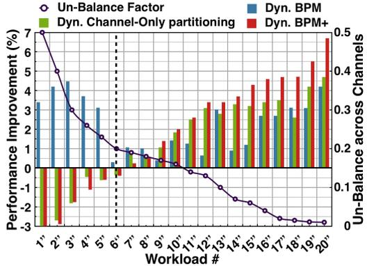
Figure 12. Dynamic Partitioning's performance under different unbalance factors.
