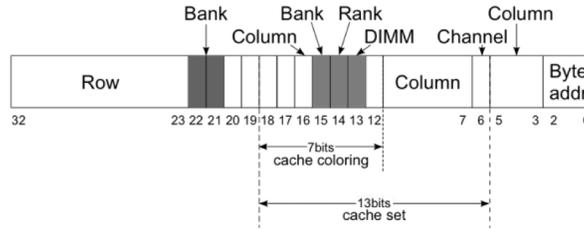
Figure 2. Address mapping policy of our platform (i7-860 8GB DDR3). The bank bits are divided into two separate parts. One is overlapped with cache set bits and the other is independent.
