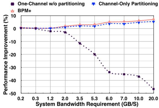
Figure 5. The correlation between bandwidth demands and performance changes caused by different policies. (This figure includes tens of workloads. The baseline is channel interleaving).
