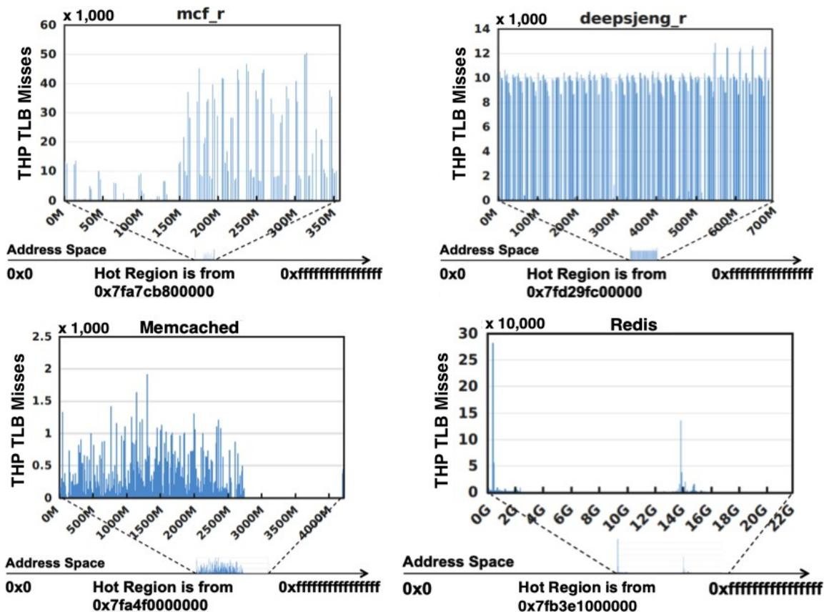
Figure 1: The number of TLB misses of Huge Pages for 4 applications in a 5-seconds sampling window.
