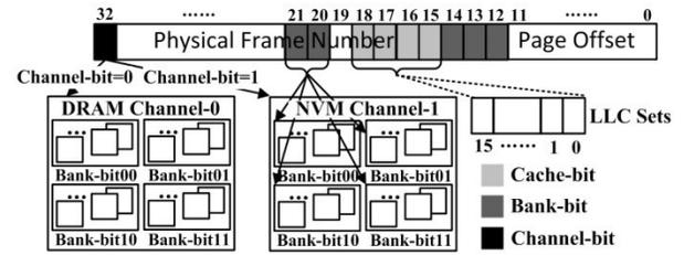
Fig.2: Address mapping across cache-channel-bank of full hierarchy vertical management for hybrid memory system. Based on Intel i7-860.
